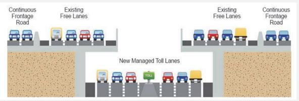
Cross section at cut and partial cover echoes the scope of I-70 East
